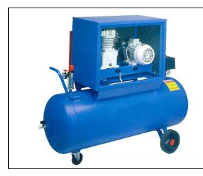
Machine used for the production of compressed air. It consists of a piston compressor with power supplied by an electric motor, a refrigerator and a tank. Its working principle is air compression: air is taken from the atmosphere, compressed by the compressor and collected into a tank. A filter is fitted at the intake to prevent foreign particles from going into the cylinder head. A cooling coil removes the condensate created by the heating of compressed air.
