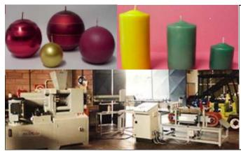
Extrusion machines and presses are used in the industrial production of candles.
