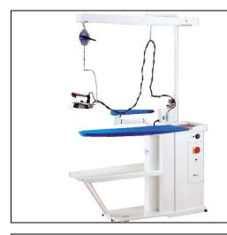
Integrated industrial ironing boards for the final finishing of clothing. The appliance is equipped with iron, vacuum blow table and sleeve form board. Ironing boards, utility presses and spotting tables make up an ironing group for various operators. Each machine can be self contained or connected to a steam, vacuum and compressed air set.
